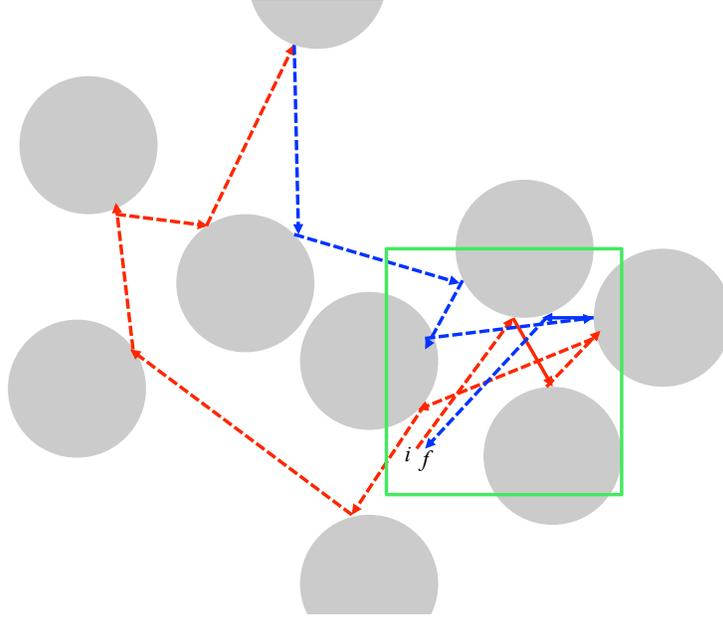
**Figure 5.** In this figure we depict a class of paths whose initial and final stages are strongly correlated. In the green box, red trajectory (outgoing) and blue trajectory (incoming) feel the same potential and the diffusive description does not apply here.
