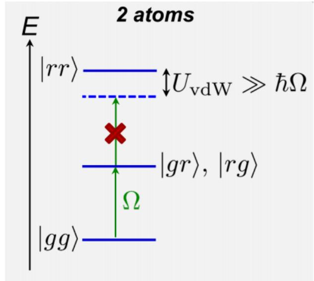
Figure 2: Blockade regime for Rydberg atoms. Two atoms placed close to each other cause the Rydberg level to be shifted up by the Van-Der-Waals interaction, meaning they cannot both be simultaneously excited by the same light field. Image from [13].
